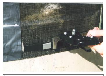
7. Thread the top band through the Tensioning Tool and snug the pusher bar against the clip. Squeeze the handles to tighten the band as much as possible.
