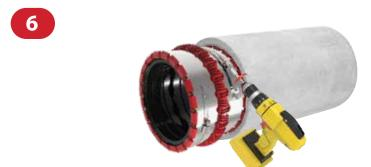
When the coupling ID's are closely matched to the pipe/adaptor OD's, install the MAXADAPTOR® Coupling onto the ShuvlNose® Adaptor. Take up all slack in coupling with a cordless drill or socket wrench.
