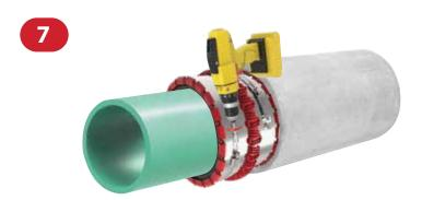
Insert the smaller pipe into the MAXADAPTOR® Coupling and take up all slack in coupling with a cordless drill or socket wrench. Complete the installation by tightening the tension clamp, alternating back and forth, to 80 in/lbs. minimum torque.
