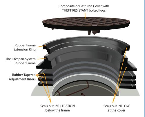
All components are made from impact-dampening, sound-absorbing, corrosion-proof, ultra-high-density virgin rubber material.
